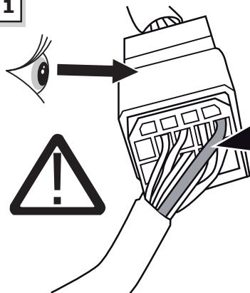
Please check if B+/30 permanent power wire in trailer preparation connector has got a minimum diameter of 1,5 mm<sup>2</sup>. If less than 1,5 mm<sup>2</sup>, continue with Option 2!
