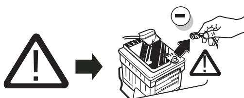
Note: It may be necessary to check if this vehicle has a stored radio code before disconnecting the battery!
