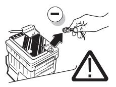
Disconnect Batterie to reset PDC-ECU!
