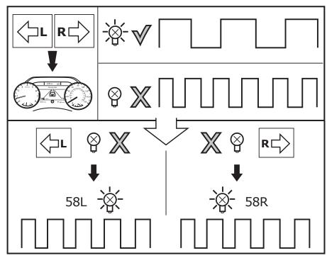
In case of trailer turn indicator failure:
