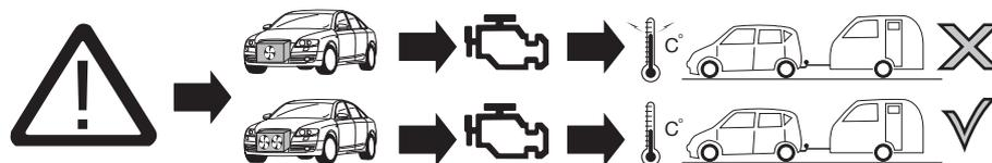
**ATTENTION!** The vehicle's cooling capacity may have to be increased when retrofitting a trailer coupling! You must observe the manufacturer's instructions!!
