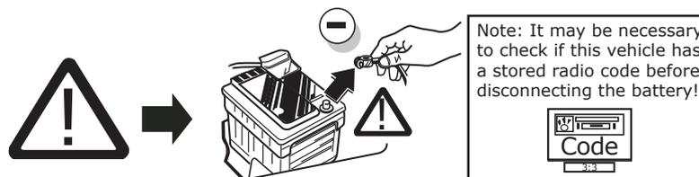
**ATTENTION!** In order to avoid mal-functions and damage to the vehicle's electrical system the earth terminal **must be disconnected** from the vehicle's battery **before starting work!**
