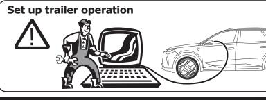
The light functions on the trailer will only operate <u>AFTER</u> the vehicle has been re-coded!
