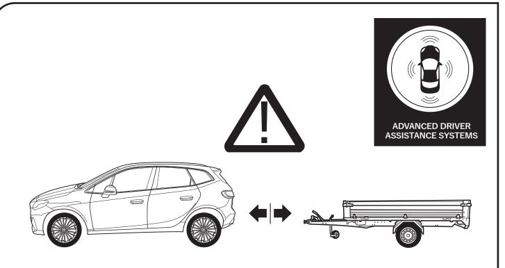
This kit does not support any of the assistance systems of the vehicle. Vehicle assistance systems may have to be deactivated manually when towing a trailer!
