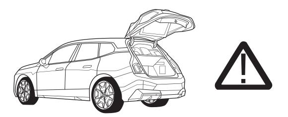
Please note that the operation of the electric tailgate will continue to function with a bicycle carrier/trailer/caravan attached. It must be operated manually.
