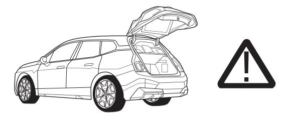
Please note that the operation of the electric tailgate will continue to function with a bicycle carrier/trailer/caravan attached. It must be operated manually.
