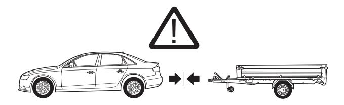
This kit does not support any of the assistance systems of the vehicle. Vehicle assistance systems may have to be deactivated manually when towing a trailer!
