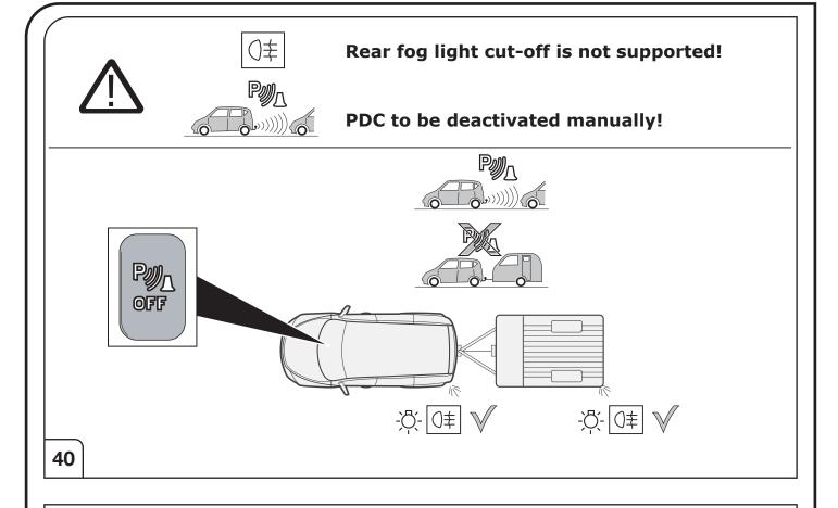
The following light functions for the trailer are not **supported** by all towing vehicles **with DRL circuit:**
